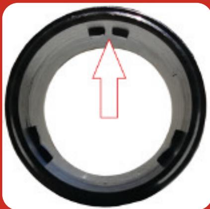
The adapter ring has three locking lugs on the inside of the ring. One locking lug has a position groove. There is a locking guide on the connector. Place the ring so that the position groove of the ring fits into the guide of the plug with the lug and turn it clockwise by 90°.
