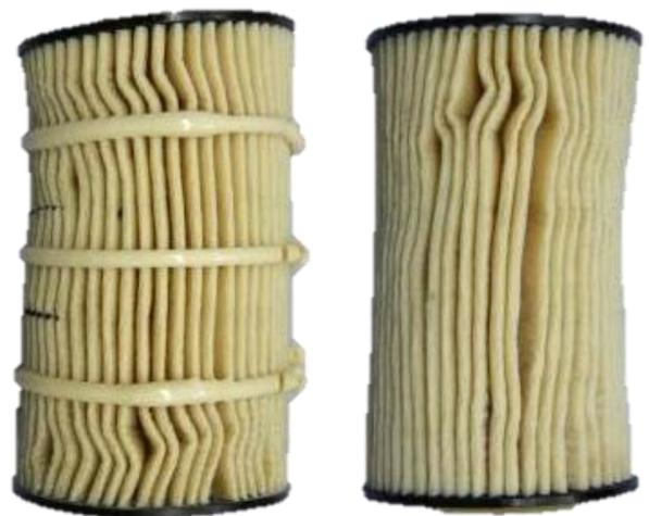
Both filters have been pressure and performance tested. Picture shows collapse pressure test whereby both filters show same structural and visual damage. Glue beads break after 2bar of pressure.
