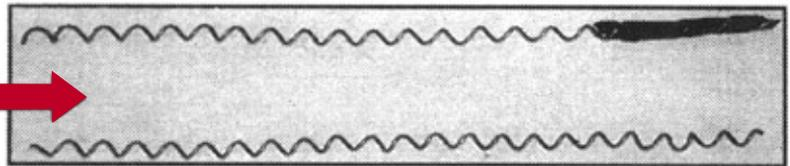
If contaminants accumulate on the turbolator, the corrosion process will interrupt for a short time and the blockage build up higher pressure, which causes a really fine stream of refrigerant under high pressure and creates holes in the U-arches.
