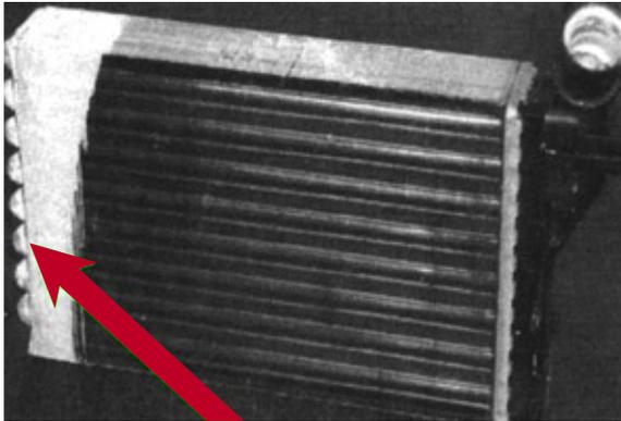
By cars with integrated turbolator heaters the rate of failure by leakage after an exchange increases.
