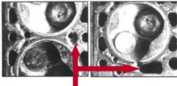
**Picture 4 + 5 (top right) shows the cylinder head top with the affected by using to less or wrong frost protection. The released metallic contaminant circulates in the cooling system and blocks the little openings as the U-arches in the heater.**
