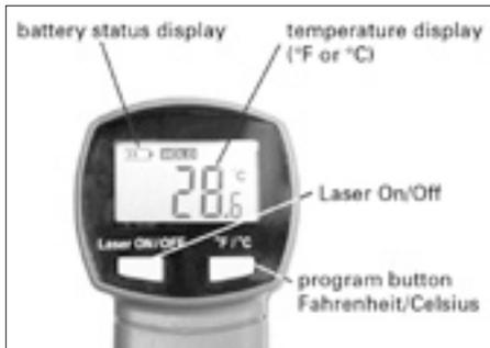
Fahrenheit/Celsius programme button: This button can be used to switch between °C (Celsius) and °F (Fahrenheit). Laser ON/OFF: This button switches the laser on or off.
