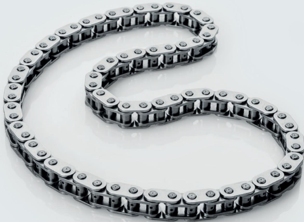
Briefly explained, this technology uses physical vapour deposition (PVD) to create a chromium nitride layer on the respective component surfaces. It ensures that the chain links can withstand wear and the chain as a whole is resistant against elongation, thus contributing to an even longer service life of the timing chain.
