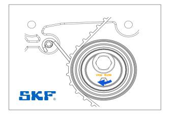
6. Maintain adjustment dial with the Allen key to torque tensioner bolt to 49 Nm.
