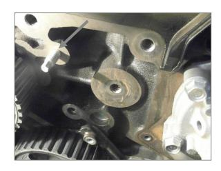
2. Set the coil spring on the stud mounted previously. Fit the SKF tensioner VKM 15218.
