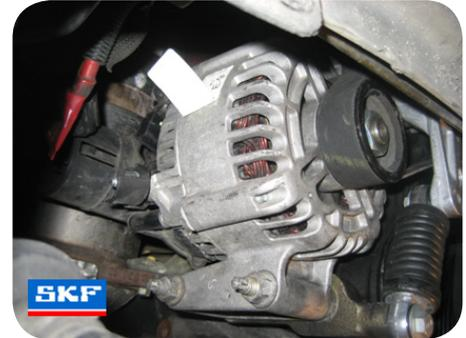
3. Remove the alternator bracket with the VKM 34032 tensioner attached to it.
