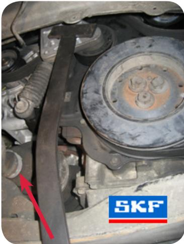
1. Release the tension from the multi-v belt, by attaching the correct tool (Ford T303676) to the captive nut on the back of the VKM 34032 tensioner.
