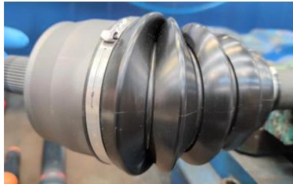
The new design of the wheel-side CV-Joint boot allows the boot to keep its characteristics even with the highest steering angles, leading to a reduced stress and longer life for the boot itself.
