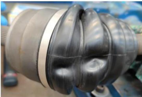
**NEW DESIGN:** suitable for high steering angles.
