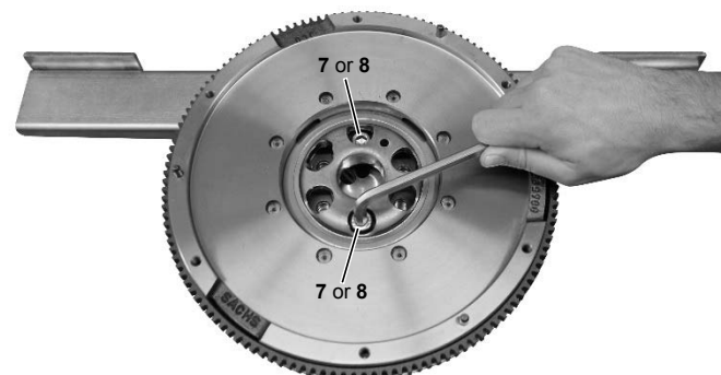
Fig. 13: Fasten DMF to base plate "1.2".
