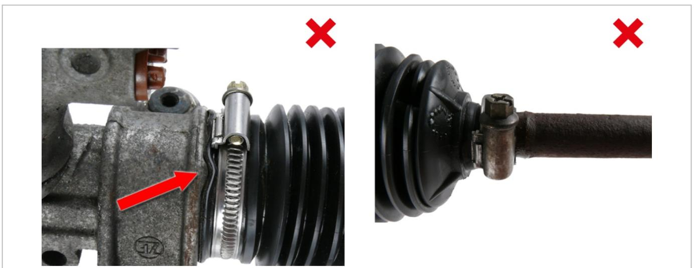
Fig. 7: Bypass: faulty sealing with hose clamps
