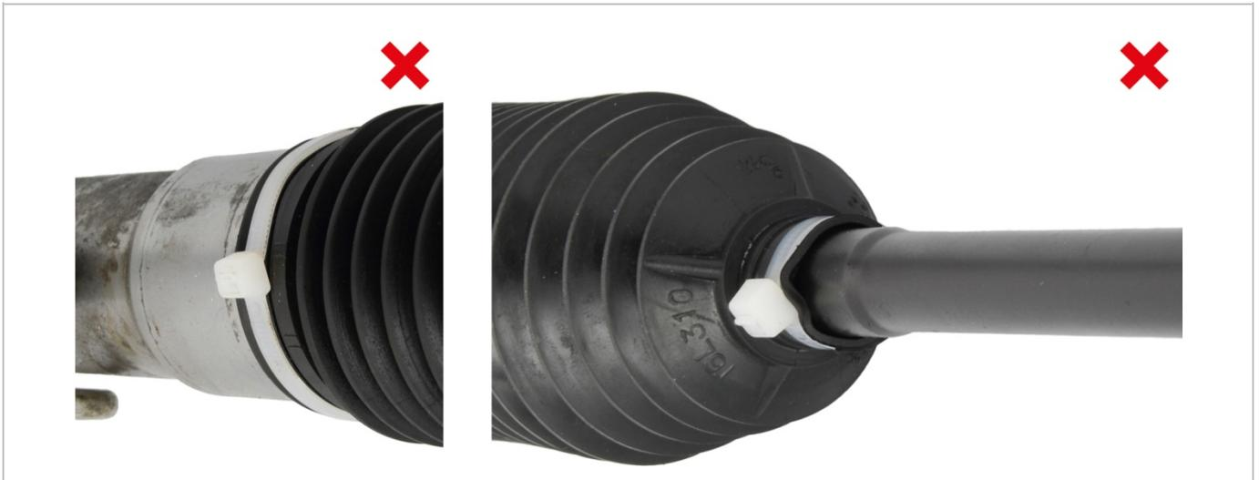
Fig. 8: Bypass: faulty sealing with cable ties
