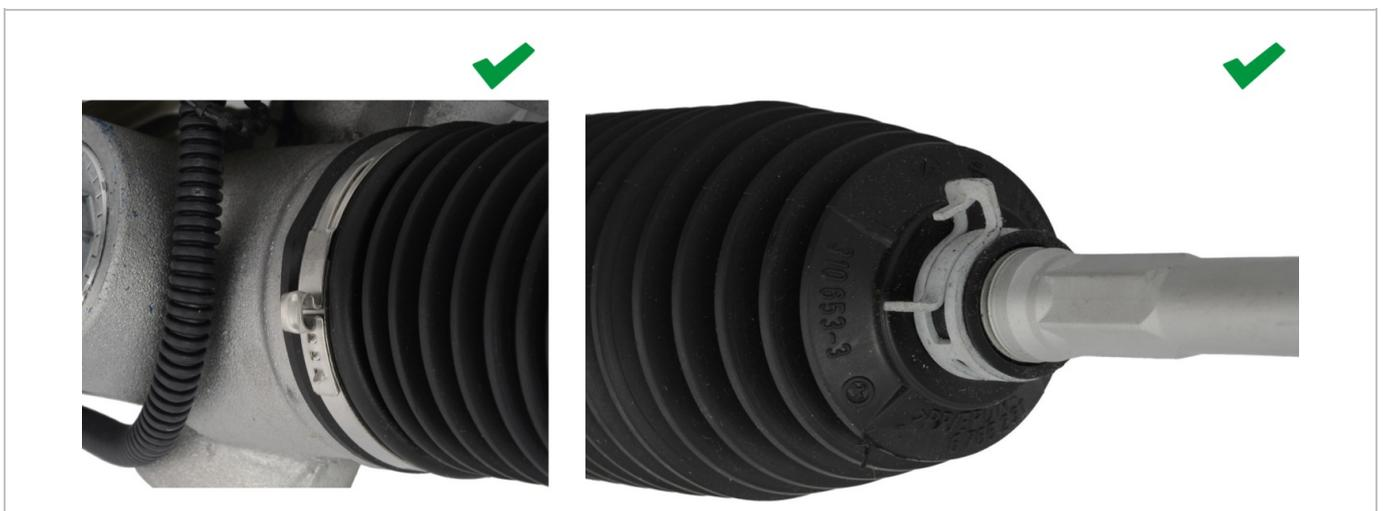
Fig. 6: No bypass: correct sealing with metal clamps
