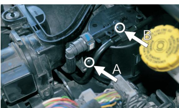
**EN** Fix battery cover (A), air filter cover (B), start engine, check fuel system for leakage, install engine masking frame
