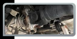
The reason for this may be a faulty or worn universal joint. This may result in complete failure of the power train. Always replace the joint if in doubt.
