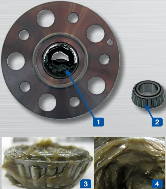
**EN** When fitting this wheel hub onto the stub axle, the grease (1) which the wheel hub is filled with is squeezed out. Generously grease the outer taper roller bearing (2) and the bearing shell before fitting the bearing (3 and 4).
