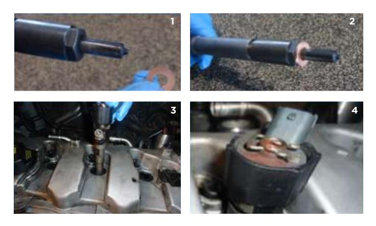
2 After inserting the injectors move the bolt to the forward position for the barrette to hold the injector. In that position it is possible to tighten the bolt with a torque of 26 3 2 Nm.
