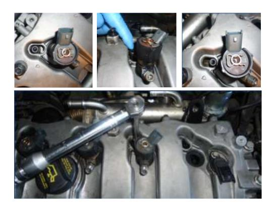
2 Finally, fit the caps for the holes of the retaining bolts with the new gaskets.
