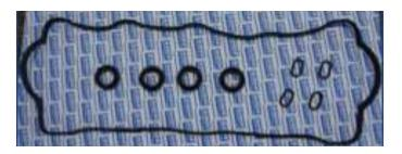
2 For the installation of the new injector oil seals will use the special tool that allows us to put them level and positioned correctly. Then place the gasket in housing without applying any sealant in this section.
