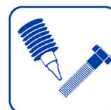
**5.** To join the components and to put the bolt before **15-25 minutes** after product application.
