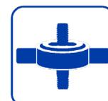
**3. Regarding bolt housing**, to clean the thread surface using a tap tool with the same metric and pitch as bolt. To extract the dirt, blowing or vacuuming inside bolt housings.
